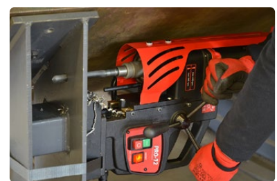
Drilling capacity up to 25 mm (1") Lightweight design of 18 kg (40 lbs) only
