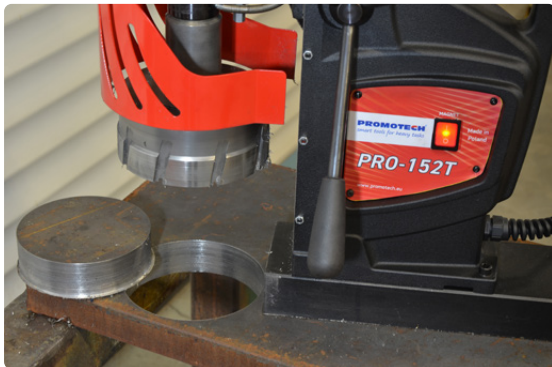
Milling capacity up to 150 mm (5-7/8")
