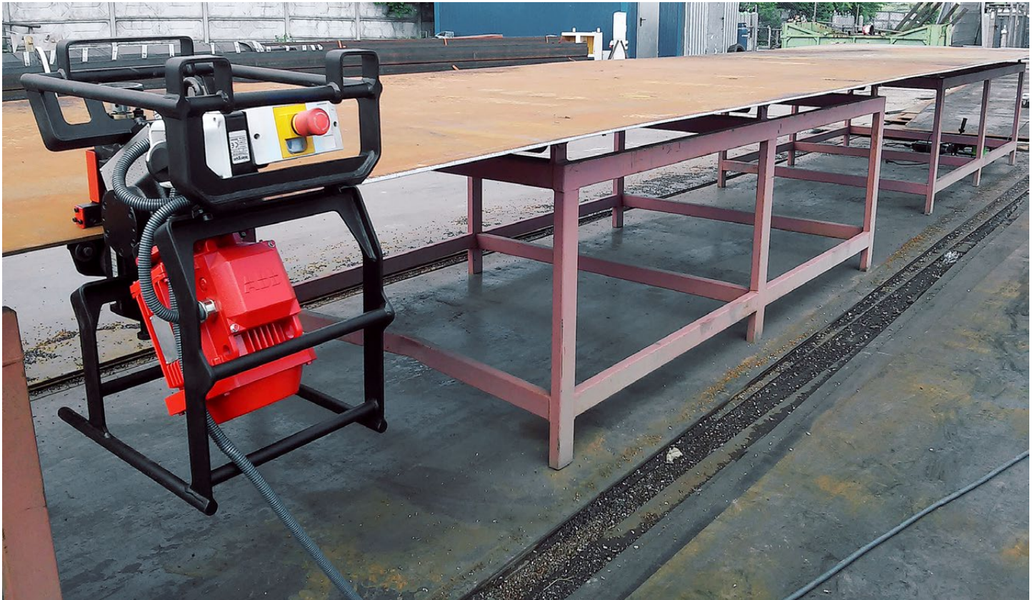
ABM-14 runs along a plate automatically
