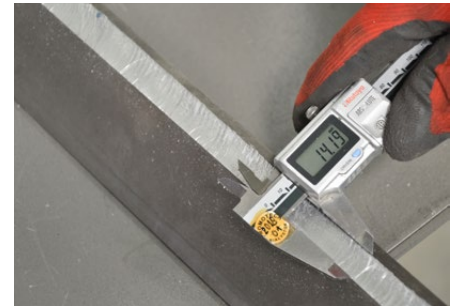
Maximum bevel width up to 14 mm
