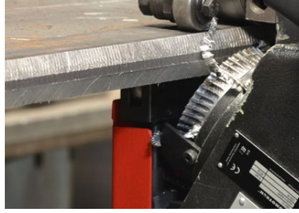
Bottom plate beveling
